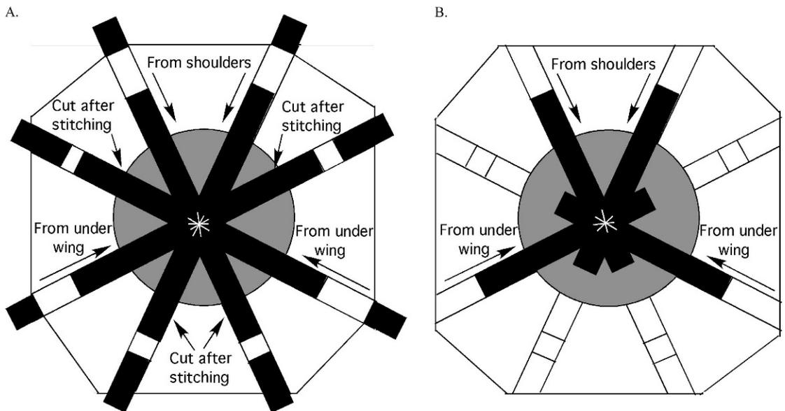
Figure 1. (A). Diagram of template for telemetry harness fitting with straps held in position and stitched. The straps coming over the shoulders and under the wings secure the transmitter on the bird. (B). Diagram of the template with the loose ends of the straps cut off. At this point the template is cut away and removed from the bird.
